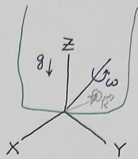
$$-\bar{\nabla}p + \bar{\rho}\bar{g} = \bar{\rho} \overline{\bar{\omega} \times \bar{\omega} \times \bar{n}} - (1)$$
