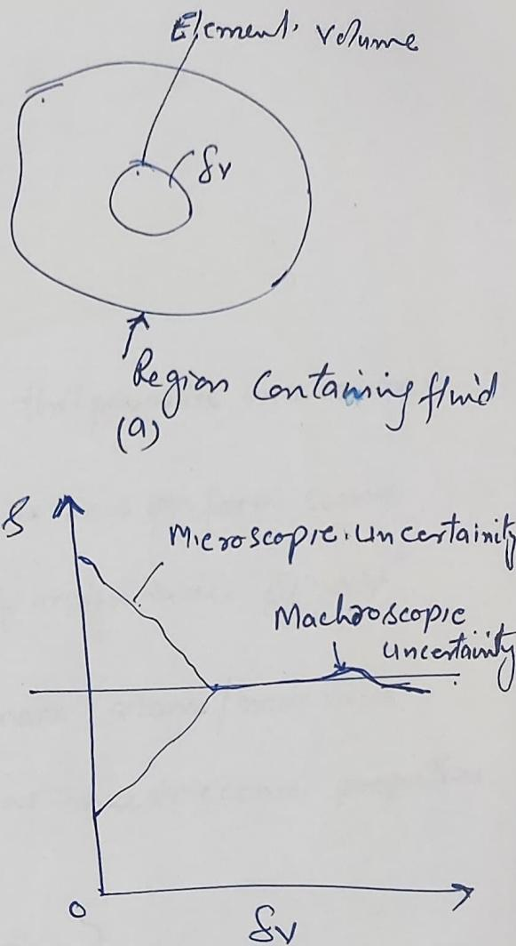
where the density as calculated from molecular mass  $\delta m$  with in a given volume  $\delta v$  is plotted versus the size of the unit volume. There is a limiting volume  $\delta v^*$  below which molecular variations may be important and above which aggregate variations may be important. The density  $\rho$  of a fluid is best defined as
