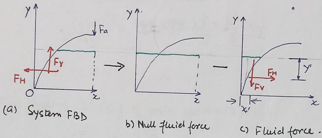
An equivalent system of fig(a). is suggested in fig. (b) & (c). The mag. & location of  $F_v$  are given by the weight and location of the centroid of the fluid above the gate; similarly for  $F_H$  are given by that of the force on an equivalent vertical flat plate.
