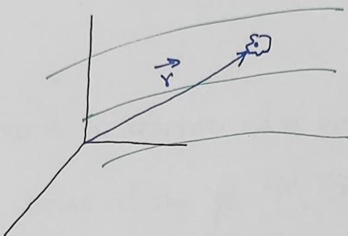
The figure shows a fluid particle at  $(\vec{r})$  at some time 't'
