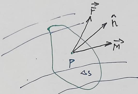
The objective is to arrive at a mathematical description of surface forces at the pt 'P'. The surface forces must be acting at each and every point of the surface in different directions. However, we know from previous Applied Mechanics course that a system of distributed forces can always be reduced to a single force  $\vec{F}$  and a moment  $\vec{M}$  at the given point 'P'.
