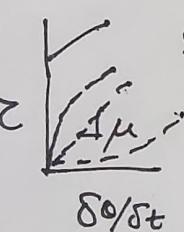
$$d\theta = \frac{du}{dy} dt \quad \text{or} \quad \frac{d\theta}{dt} = \frac{du}{dy}$$
