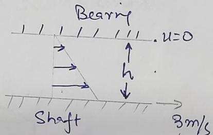
$$\frac{dy}{dx}_{\text{shaft}} = \frac{u_b - u_s}{h}$$
